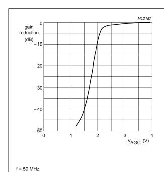
Fig.5 Gain reduction as a function of the AGC voltage; typical values.
