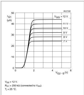
Fig.16 Gate 1 current as a function of gate 2 voltage; typical values.
