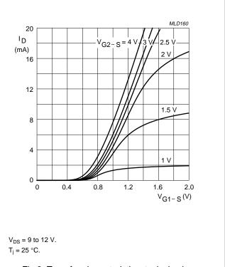
Fig.8 Transfer characteristics; typical values.
